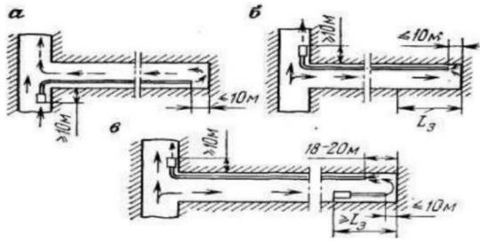
The main methods of ventilation of horizontal mine welds with the help of fans and pipes.
