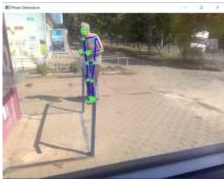
Figure 2: User interface of the human recognition program in a collaborative robot-manipulator working area
