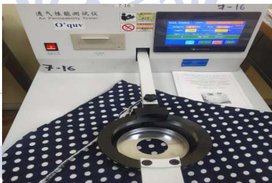
2-rasm.Suprem trikotaj matosining havo o'tkazuvchanligini tekshirish jarayoni.
