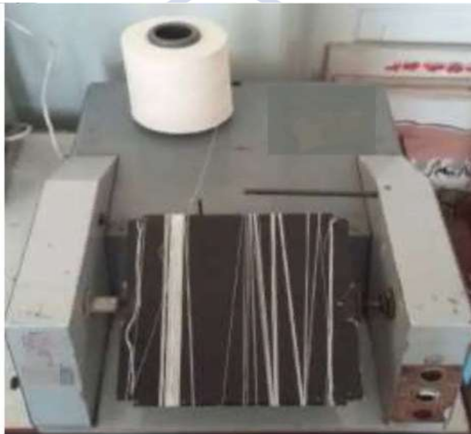
Figure 1. An image of the MOK device that determines the cleanliness of the thread.
