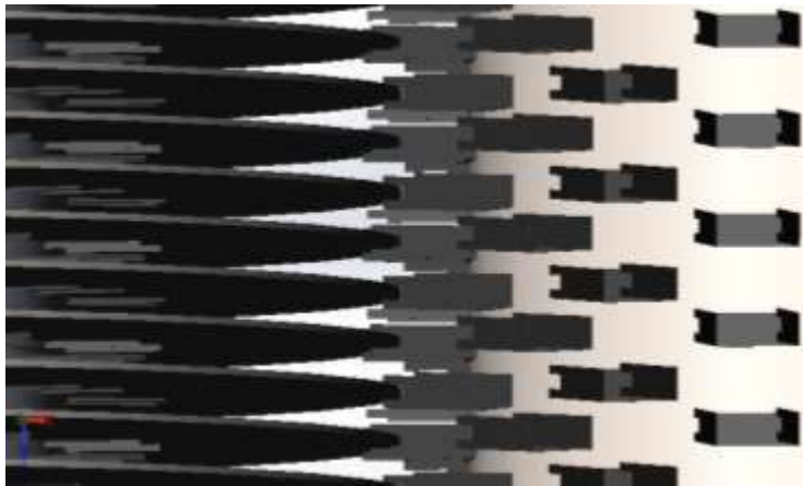
Figure 3. A view of a device that removes cotton fiber from saw teeth using a brush drum with a saw cylinder
