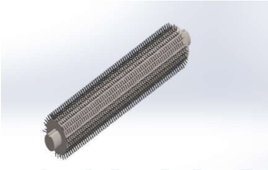
Figure 1. 3D view of a device that removes cotton fiber from saw teeth using a brush drum.
