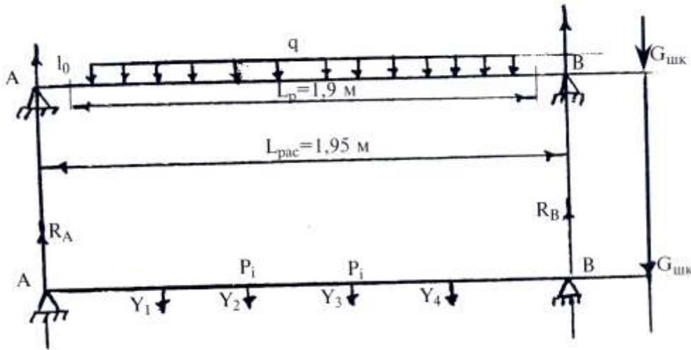
Figure 5. Calculation scheme of the drum
