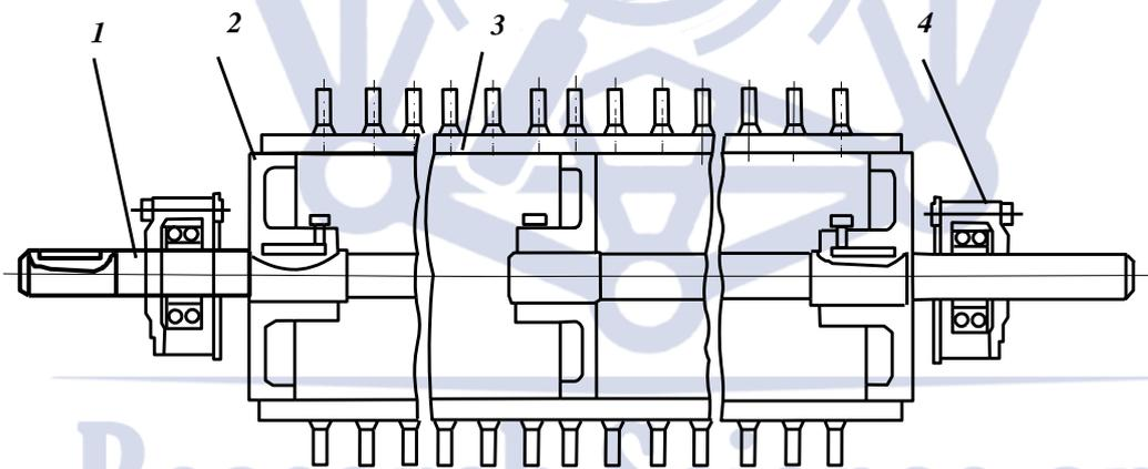
Figure 4. Cross section of an improved pile drum; clipping scheme
