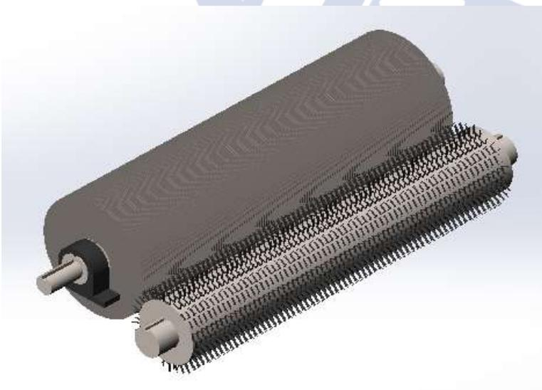
Figure 2. A view of a device that removes cotton fiber from saw teeth using a brush drum with a saw cylinder.
