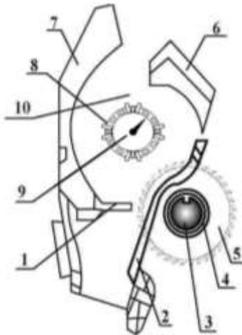
Figure 1. The working chamber of the saw demon
