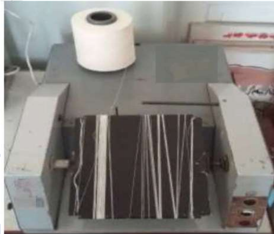
Figure 1. Illustration of the NOC device for determining the purity of yarn.
