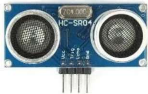
Figure 1: General view of the HC-SR04 sensor
