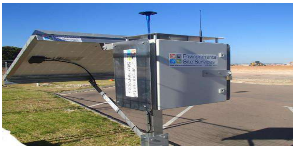
Figure 2. Air Quality Monitoring Station
